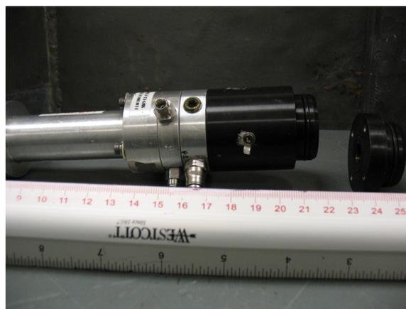
A solid target plate was prepared which had a hole drilled in the top to allow a temperature probe to be inserted to the middle of the plate. This enabled the temperature of the target plate to be monitored between the beam spot and the water cooling on the back of the plate.
