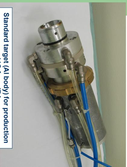
Standard target (Al body) for production  $^{11}\text{C}$  from IBA
