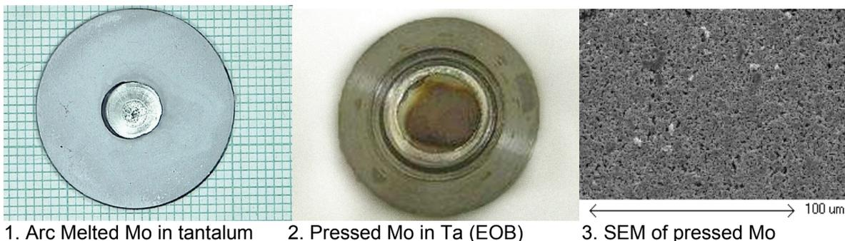
**$^{99m}\text{Tc}$  Production:**  $^{99m}\text{Tc}$  was produced via the  $^{100}\text{Mo}(p,2n)^{99m}\text{Tc}$  nuclear reaction on a 19 MeV medical cyclotron using an incident proton energy of 15-17 MeV at current between 14-52  $\mu\text{A}$ . After bombardment targets were subjected to electrochemical dissolution,  $^{99m}\text{Tc}$  was purified by ion-exchange chromatography and recovered as pertechnetate.
