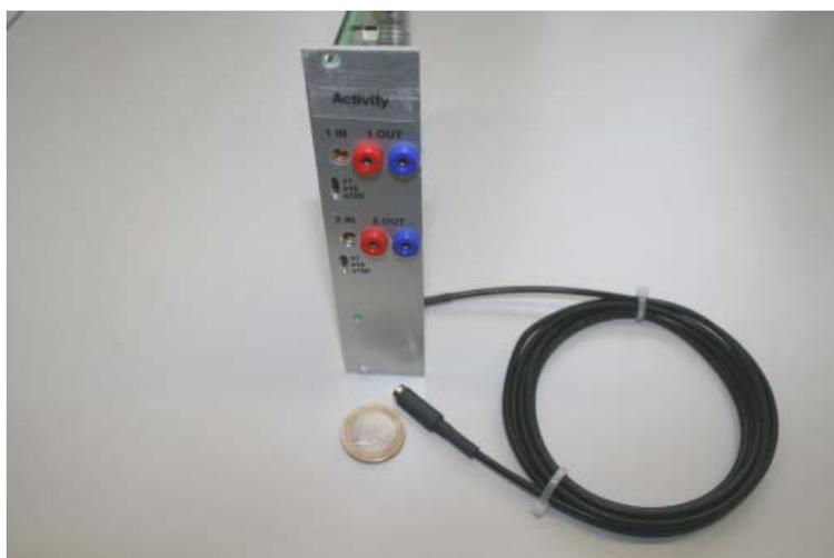
Fig. 3 Amplifier with photodiode radiation detector
