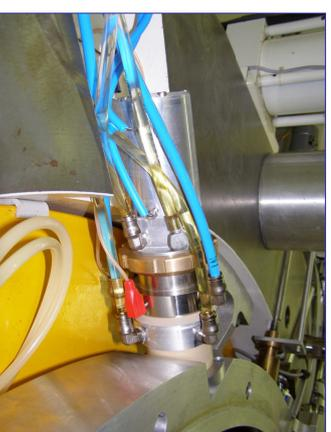
$[^{18}\text{F}]\text{F}_2/[^{18}\text{O}]\text{O}_2$ -gas target
