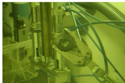
Fig 2: Broken Ga Target
